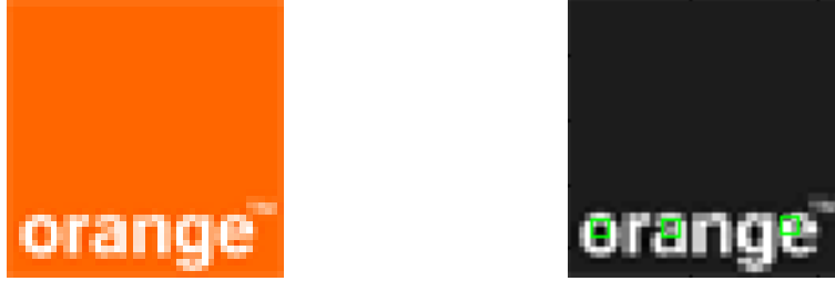
Figure 6: A logo not suitable for SIFT matching. The logo, as it appears online, lacks enough detail to generate a reliable set of feature points for matching. On the left, the logo; on the right, the logo as processed by our system, with SIFT keypoints in green.
