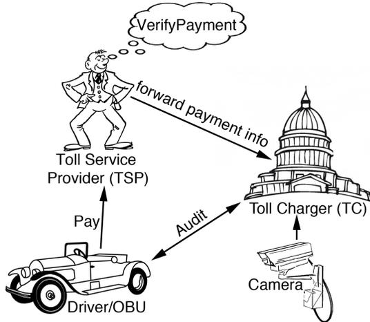
**Figure 1:** An overview of how the Milo system works. As we can see, the OBU deals with the TSP for payment purposes (using the Pay protocol), but for spot checks it interacts with the TC (using the Audit protocol). The TC conducts these audits using both the information recorded by the cameras it operates along the roads and the OBU’s payment information, which is forwarded on from the TSP after it has been checked to be correct (using the VerifyPayment protocol).
