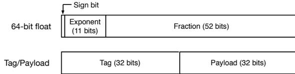
Fig. 1. Illustration mapping the bits of an IEEE 754 double precision floating-point number to the tag and payload portions of a 32-bit JSC JS value.
