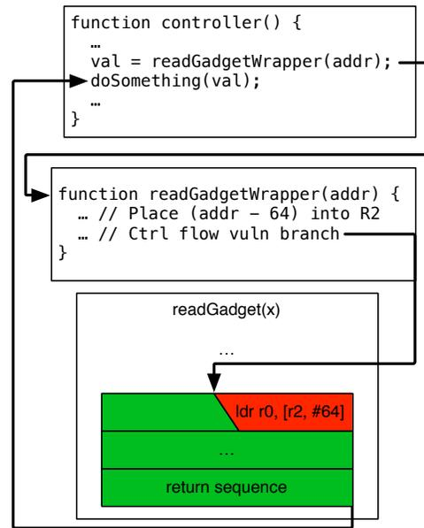
Fig. 4. Diagram of the invocation of the read gadget with arrows showing control flow.
